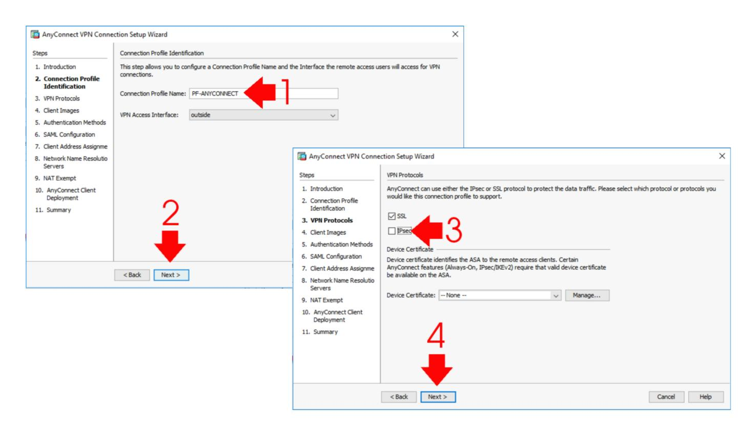
Install Ssl Certificate Asa Firewall Connection
